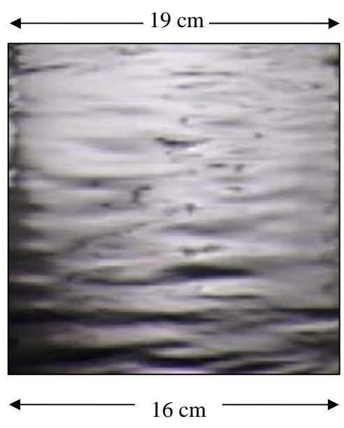
Figure 2.12 Free-surface texture for flow over smooth flat bed with flow depth of 8 cm with illumination from upstream. Camera was placed downstream of the channel with 30°-angle from horizontal.
